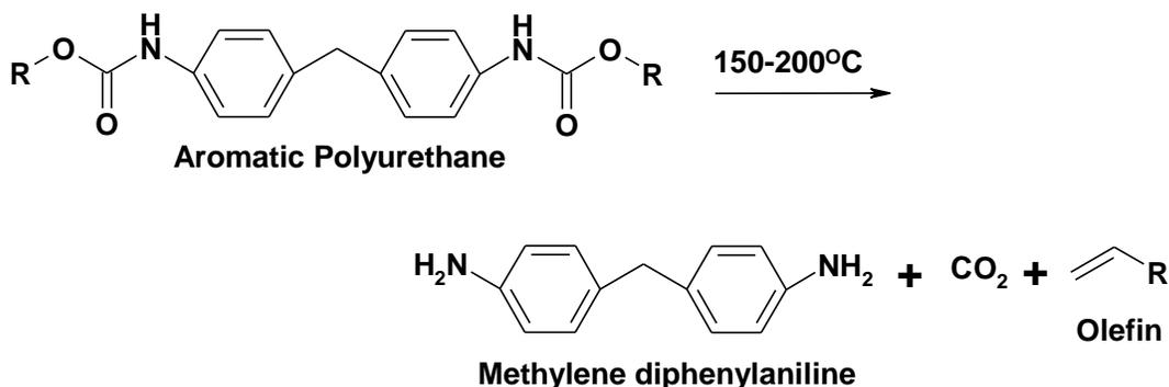
**Figure 4.** Thermal degradation of aromatic polyurethane, resulting in formation of toxic dimethylaniline.
