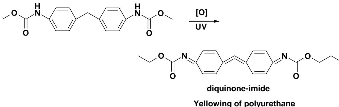
**Figure 3.** Formation of the diquinone-imide structure responsible for yellowing of polyurethane in the presence of ultraviolet light.
